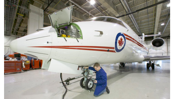
A non-destructive testing technician, certified by NRCAN, conducts an ultrasonic inspection to check for cracking around bolt holes in the landing gear of this CC144 Challenger aircraft.
